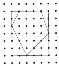
The area of the figure is the area of the rectangle  $5 \times 6 = 30$  less the four triangles on the corners, that is,  $30 - \frac{1}{2} \times 2 \times 1 - \frac{1}{2} \times 3 \times 1 - \frac{1}{2} \times 3 \times 3 - \frac{1}{2} \times 2 \times 4 = 30 - 1 - 1\frac{1}{2} - 4\frac{1}{2} - 4 = 19$  square centimetres,
